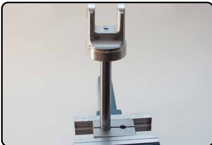
Clamp the piston-rod in clamping block T1202S.
