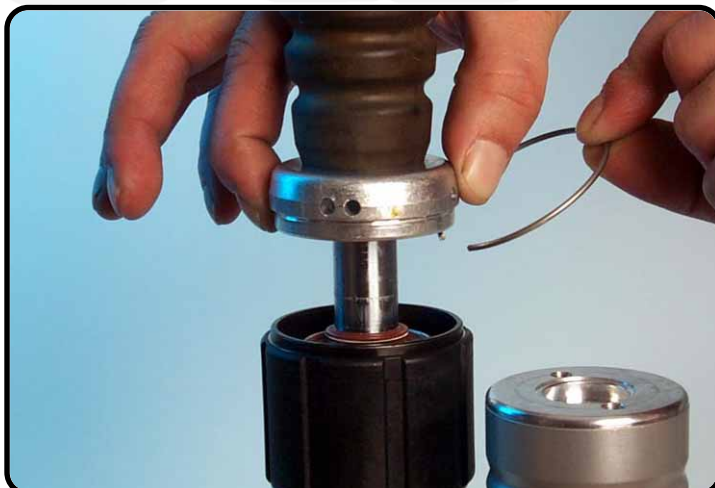
Assemble the springring.
