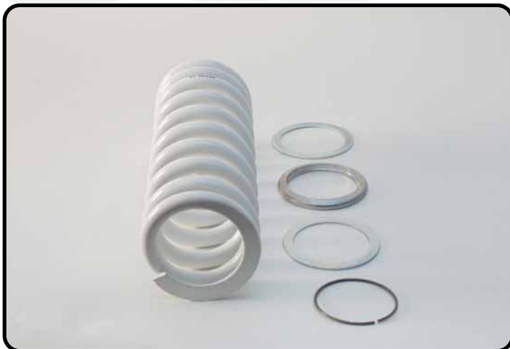
Spring with washers, spring retainer and springring.
