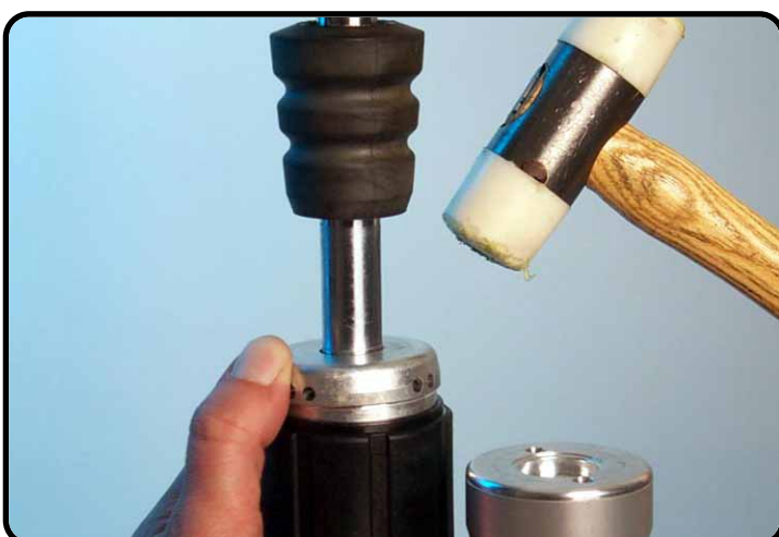
Tap the cap into the tube.
