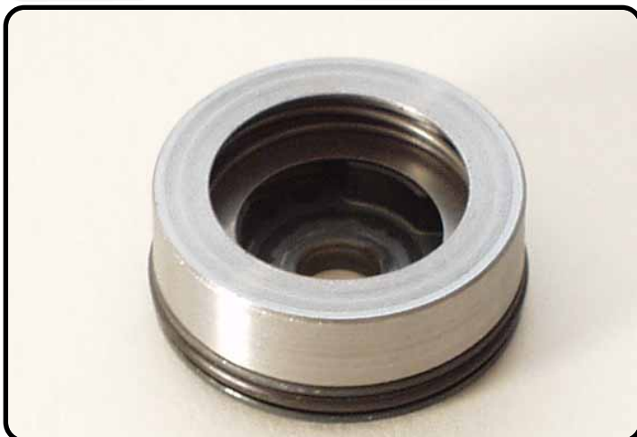
Piston with the check-valve side.
