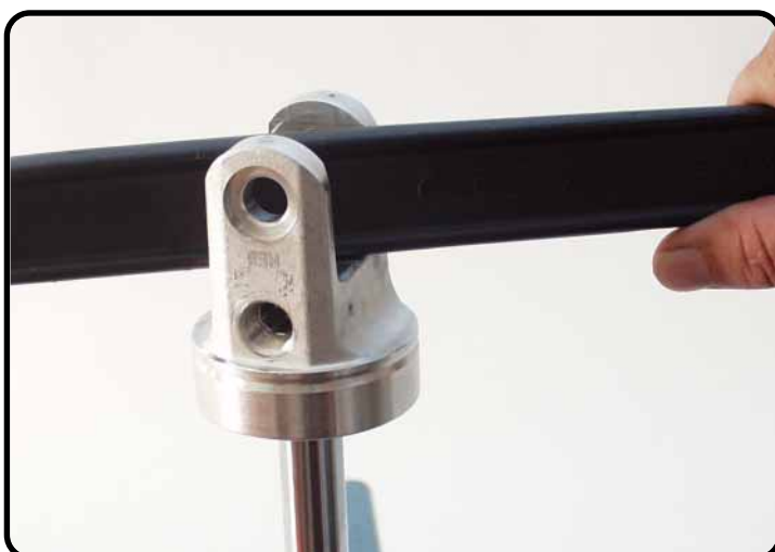
Unscrew the mounting-fork.
